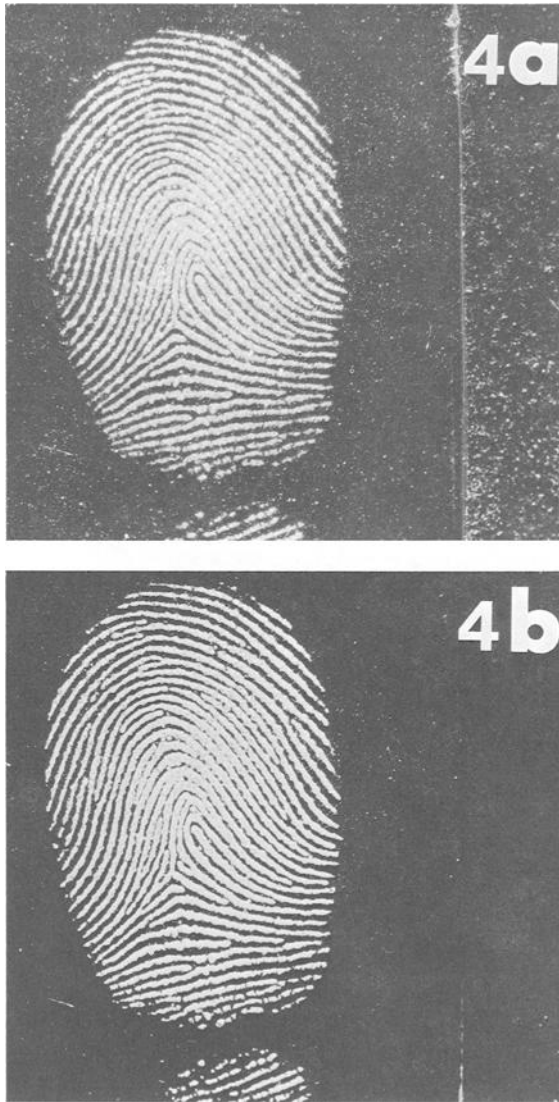
FIG. 4—Fingerprint on aluminum foil developed under laser first by dusting (a) and again after subsequent glue treatment (b). Photographs made under equal conditions, excepting exposure time, 30 s for a and \frac{1}{4} s for b.
