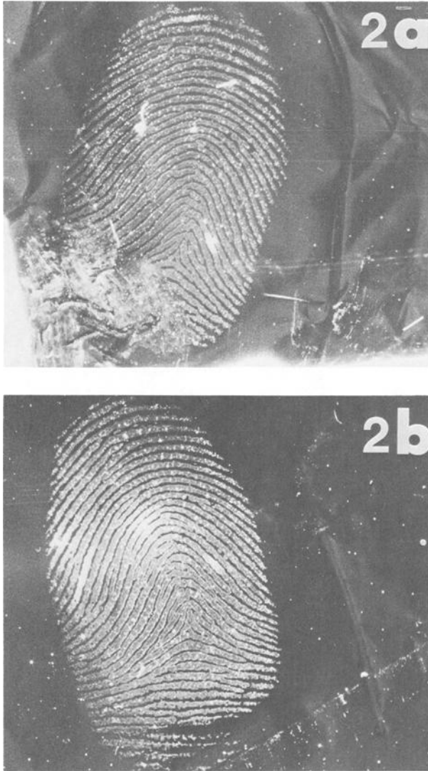
FIG. 2—Fingerprint on aluminum foil developed under blue-green argon-ion laser first by inherent fluorescence (a) and then by glue treatment (b).
